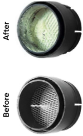
The before/after effect on a small mesh shows the degree of pollution after 90 minutes of soldering.
